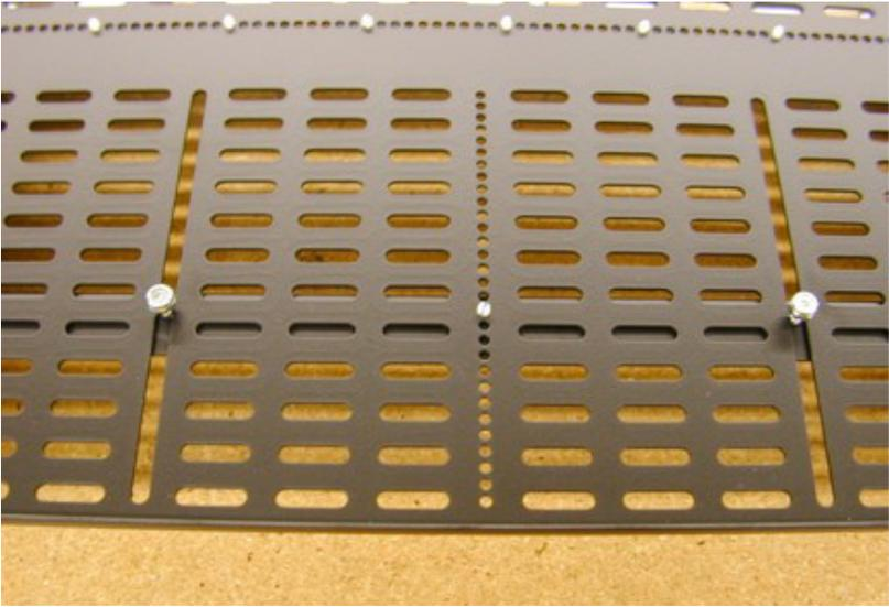
5. Once the pins are pressed in, turn the unit over and thread on the **Nylon Locking Nuts** as shown above until they are tight.
