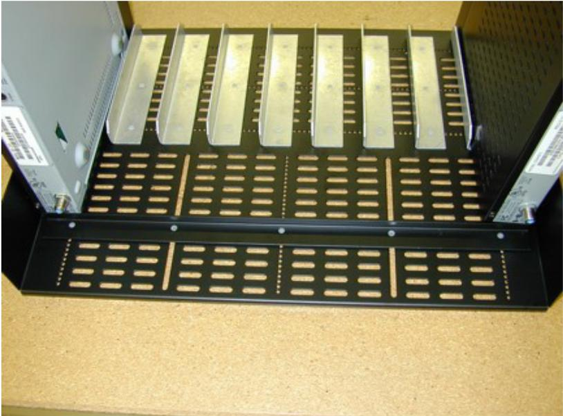
3. Keep in mind the front of the receiver should not extend passed the mounting tabs on the front of the shelf, as this is critical for proper mounting in the Head-End rack.
