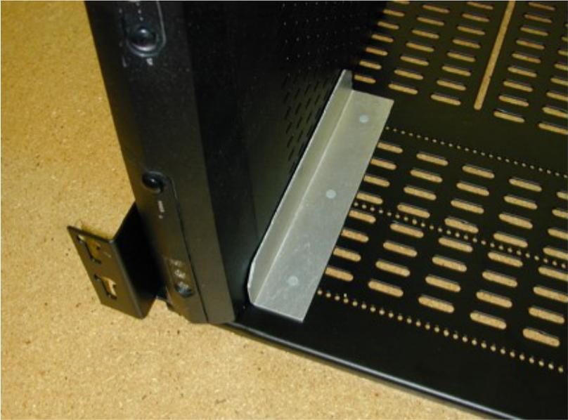
3. Place a **Dividing bracket** close to the receiver while still being able to align it and press one snap pin into a aligning hole, align the divider and press in the other two pins. Keep in mind to leave enough room for the feet of the receiver.
